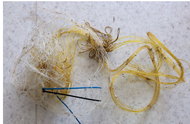
Figure 21. Net samples retrieved from Location 2 after 25 months of submergence. PBSAT samples were entangled (left).
