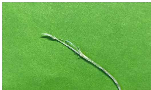
Figure 23. Frayed fracture of PBSAT fiber from Location 2 after 25 months of submergence.
